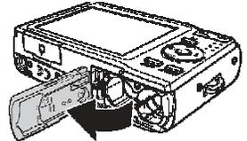
3. Insert the batteries into the compartment with the terminal facing inside the camera and the battery indent next to the compartment door.
